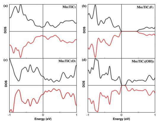
Fig. 3 Calculated total density of states (DOS) of perfect MXenes. (a) Pristine MXene, (b) Mo<sub>2</sub>TiC<sub>2</sub>F<sub>2</sub>, (c) MoTiC<sub>2</sub>O<sub>2</sub>, and (d) Mo<sub>2</sub>TiC<sub>2</sub>(OH)<sub>2</sub>. Black and red lines show spin-up and -down states, respectively.
