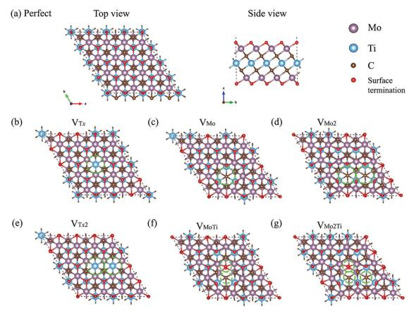
Fig. 1 Fully relaxed structural models of different types of defects considered in monolayer ordered  $Mo_2TiC_2T_{x\cdot}$  (a) Top and side view of the perfect MXene. Top views of (b)  $V_{T_{uv}}$  (c)  $V_{Mov}$  (d)  $V_{Moov}$  (e)  $V_{T_{uv}}$  (f)  $V_{MoTi}$ , and (g)  $V_{Moov}$  (ii)  $V_{Moov}$
