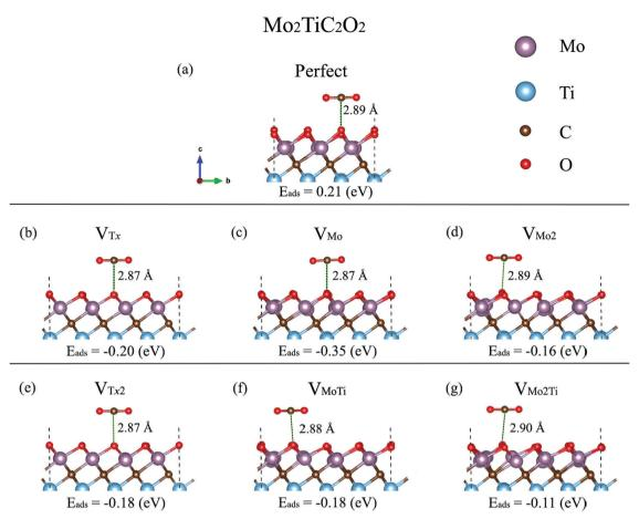
Fig. 5 Relaxed adsorption configurations of a  $CO_2$  molecule on the perfect and defected  $Mo_2TiC_2O_2$  MXene. (a) Perfect MXene, (b) MXene- $V_{T,r}$ (c) MXene- $V_{MO_2}$ , (d) MXene- $V_{MO_2}$ , (e) MXene- $V_{T_2}$ , (f) MXene- $V_{MOTi}$ , and (g) MXene- $V_{MO_2}$ Ti-
