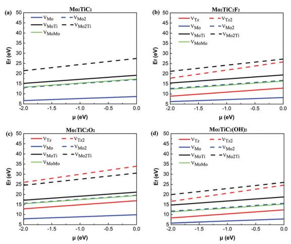
Fig. 2 Formation energies of all types of defects as a function of the chemical potential of the removed atom(s) in the range of  $-2 \text{ eV} < \mu < 0 \text{ eV}$  in (a)  $Mo_2TiC_2$ , (b)  $Mo_2TiC_2F_2$ , (c)  $Mo_2TiC_2O_2$ , (d) and  $Mo_2TiC_2(OH)_2$ .
