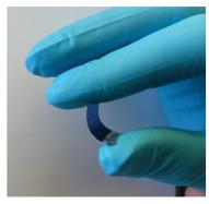
Fig. 6 A piece of flexible, thin-film silicon. (Image used with permission of Dr N. Bennett, Heriot Watt University.)
