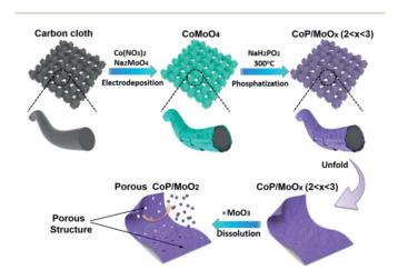
Scheme 1 Illustration of the preparation process of the porous CoP/ MoO<sub>2</sub> thin films.
