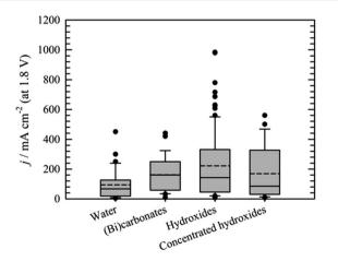
Fig. 8 Comparison of the current densities achieved at cell voltage 1.8 V using water, <sup>22,55,57,107,108,114,115,118,120,124,129,132–136,139–142</sup> (bi)carbonates<sup>54,55,96,106,114,116,122,141,143,151</sup> hydroxides<sup>55,59,93,95,101</sup>–104,109,111–114,117–119,121,123,124,126–128,132,135,136,139,141,145,146,155–159 as liquid electrolyte. Bar for "concentrated hydroxides represents KOH solutions >1 mol dm<sup>-3</sup>
