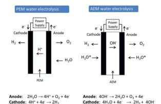
Fig. 1 Comparison of water electrolysis cells and chemistries using either a Proton Exchange Membrane (PEM) or an Anion Exchange Membrane (AEM).\* Current AEM electrolyzers use a water feed with added electrolyte  $(HCO_3^-/CO_3^{2-})$  or dilute KOH) to obtain sufficient performance. AEM electrolyzers can operate with electrolyte feed at both electrodes or in anode feed only mode.
