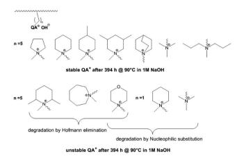
Fig. 5 Stability and degradation mechanisms of different quaternary ammonium groups tethered to a polymer backbone (PPO) by different spacer lengths as revealed by <sup>1</sup>H NMR spectroscopy. Degradation of PPO backbone in these experiments was not detected.88
