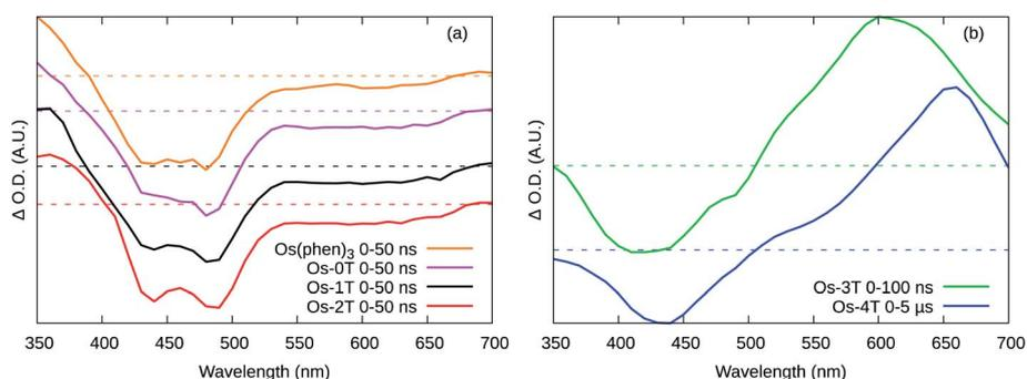
Fig. 8 Transient absorption profiles for (a)  $[\text{Os}(\text{phen})_3](\text{PF}_6)_2$ , Os-0T–Os-2T, and (b) Os-3T and Os-4T, showing the indicated integration slices.  $\Delta\text{O.D.} = 0$  is indicated by the dashed line of the corresponding color.
