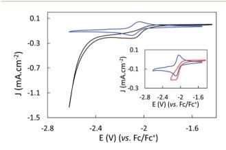
Fig. 2 Cyclic voltammograms of complex 1 under Ar (blue) and  $CO_2$  applying potentials from -1.52 V to -2.22 V vs. Fc/Fc<sup>+</sup> (red, inset) and from -1.52 V to -2.62 V vs. Fc/Fc<sup>+</sup> (black). 1 mM solution in dry CH<sub>3</sub>CN containing 0.1 M TBAPF<sub>6</sub> electrolyte; GC working electrode; The scan rate was 50 mV s<sup>-1</sup>; the second scan is shown.
