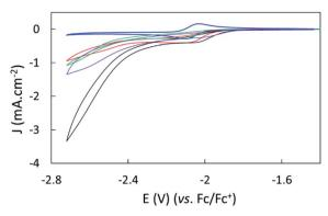
Fig. 3 Cyclic voltammograms of 1 mM complex 1 with 0.1 M TBAPF<sub>6</sub> in dry CH<sub>3</sub>CN on a GC electrode under Ar (blue), CO<sub>2</sub> (red), CO<sub>2</sub> with 0.1 M TFE (black), CO<sub>2</sub> with 0.1 M H<sub>2</sub>O (green) and CO<sub>2</sub> with 0.1 M PhOH (purple). The scan rate was 50 mV s<sup>-1</sup>; the second scan is shown
