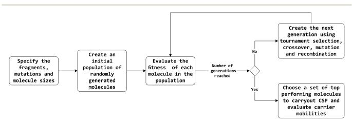
Fig. 1 High-level flow diagram of the evolutionary algorithm optimisation process.
