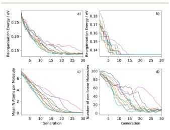
Fig. 4 Progress of the ten runs of the evolutionary algorithm, each displayed as a different colour: (a) mean reorganisation energy of the population; (b) minimum reorganisation energy; (c) mean number of nitrogen atoms per molecule; (d) number of non-linear molecules in the population. The population size was 100 in all runs.
