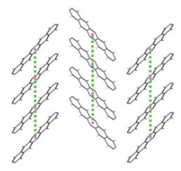
Fig. 11 A 2D plane of the global minimum energy crystal structure of 2B showing  $\gamma$ -type stacking of molecules. Red spheres mark the centroids of each molecule and the green dotted lines are the hopping pathways with the largest rate of electron transport in this crystal structure.
