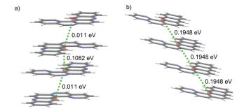
Coplanar stacking of molecules in the global energy minimum predicted crystal structures of molecules (a) 2A and (b) 4A. Red spheres mark the centroids of each molecule. Green dotted lines are the hopping pathways along molecular stacks, showing values of the electronic coupling,  $|V_{ab}|$ , after scaling.
