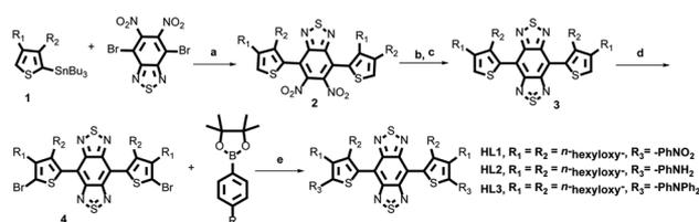
Fig. 2 The synthetic routes of **HL1–HL3**. Reagents and conditions: (a) Pd(PPh<sub>3</sub>)<sub>4</sub> and THF; (b) Zn, NH<sub>4</sub>Cl, and CH<sub>2</sub>Cl<sub>2</sub>/MeOH/H<sub>2</sub>O; (c) PhNSO<sub>2</sub>, TMSCl, and pyridine, two steps; (d) NBS, HBr, and DMF/CH<sub>3</sub>CN; (e) PdCl<sub>2</sub>(dppf)<sub>2</sub>CH<sub>2</sub>Cl<sub>2</sub> and K<sub>2</sub>CO<sub>3</sub>.
