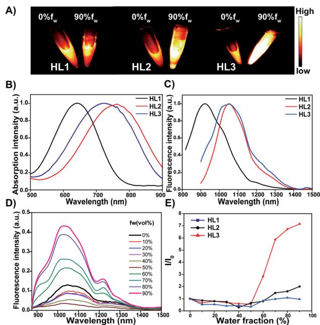
Fig. 3 (A) NIR-II fluorescence images (1000 LP, 808 nm excitation, 40 mW cm<sup>-2</sup>, and 5 ms) of HL1–HL3 in THF and THF/water ( $f_w$ , 90%); (B) absorption and (C) fluorescence emission spectra of HL1–HL3 in THF under 808 nm excitation; (D) fluorescence emission spectra of HL3 obtained upon increasing  $f_w$  from 0 to 90% under 808 nm excitation; (E) fluorescence intensity ratios ( $I/I_0$ ) of HL1–HL3 in different  $f_w$ s.  $I_0$  is the fluorescence intensity of HL1–HL3 in THF.
