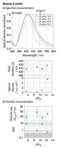
Fig. 8 Effect of initial pH (pH<sub>IN</sub>) in the growth-stage. A. UV-vis spectra, spectral peak location and optical density at the outlet of R5; B. particle size distribution (average and standard deviation) and spherical degree (RSS). Conditions: nucleation reactor → refer to Fig. 7. 5 growth reactors  $\rightarrow$  same as Fig. 6 and 7 except for changes in the pH<sub>IN</sub>.
