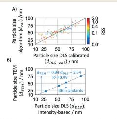
Fig. 3 A. Validation of the Mie theory-based algorithm using >100 synthesized Ag nanoparticles samples characterised by DLS. Data plotted in function of the spherical degree (RSS). B. Calibration of the DLS intensity-based particle size by TEM of commercial particles from BBi.
