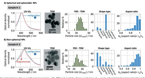
Fig. 4 Characterization of two synthesized samples with different particle shapes and sizes, A - quasi-spherical (spherical and spheroidal) particles and B - non-spherical particles, by spectral and TEM analysis. The experimental optical response (red) was compared to the estimated one using the Mie theory-based algorithm (blue).
