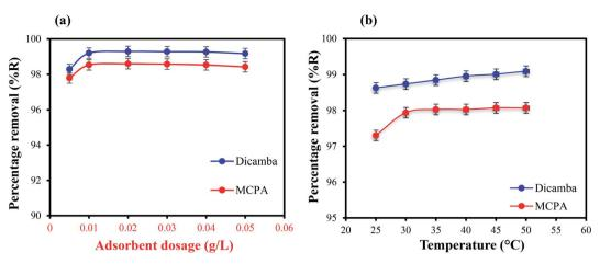
Fig. 2 (a) Effects of adsorbent dosage the red colour highlights in (a) should be black and (b) temperature on the removal of dicamba and MCPA (herbicide concentration,  $20 \text{ mg L}^{-1}$ ; equilibrium time, 25 min; rpm, 150).
