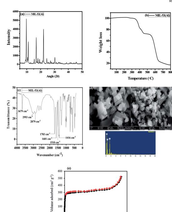
Fig. 1 (a) XRD pattern (b), TGA thermogram (c), FTIR spectrum (d), FESEM-EDX spectrum and (e)  $N_2$  adsorption—desorption isotherm of MIL-53(Al).
