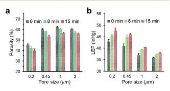
Fig. 4 The porosity (a) and LEP (b) of PP membranes with different pore size after PHDFA coating with varying deposition time.
