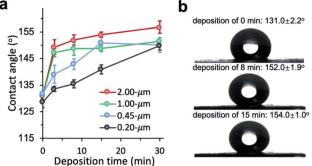
Fig. 3 (a) Effect of vapor deposition time on the wettability of PP membranes with varying pore sizes. (b) Optical images of water droplet on 2  $\mu$ m PP membranes with different deposition time.
