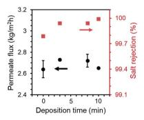
Fig. 5 Permeate flux and salt rejection of 0.45  $\mu m$  PP membranes after PHDFA coating with varying deposition time. Test condition: feed temperature at 50 °C, flow rate at 0.81 L min<sup>-1</sup>, NaCl concentration at 30 g L<sup>-1</sup>.
