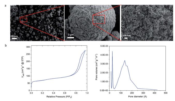
Fig. 3 Characterization of MZSM particles. (a) SEM images of the prepared MZSMs particles. (b)  $N_2$  isotherm and  $N_2$  adsorption pore size distribution of the MZSMs
