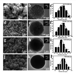
Fig. 3 SEM (a, d, g, and j) and TEM (b, e, h, and k) images and the corresponding particle size distributions (c, f, i, and l) of the YC-CaCO<sub>3</sub> nano/microspheres biosynthesized in the same concentration of yeast cell secretions (the concentrations of Ca<sup>2+</sup> and CO<sub>3</sub><sup>2-</sup> were 0.1 M (ac), 0.2 M (d-f), 0.3 M (g-i), and 0.4 M (j-l)).
