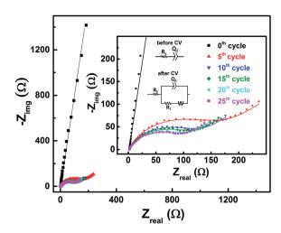
Fig. 6 EIS patterns recorded at OCP on carbon-modified GCE without rotation in 0.2 M  $\rm V^{5+}$  electrolyte after every 5 cycles. The symbols and solid lines show the experimental and the fitted data, respectively. The corresponding EC is shown in the inset.
