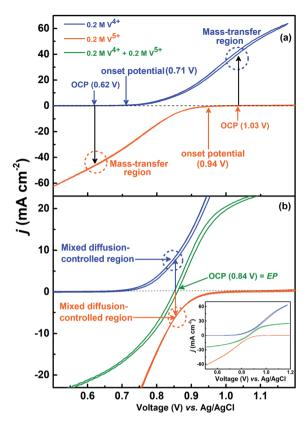
Fig. 4 CVs recorded on carbon-modified GCE at 20 mV s $^{-1}$  scan rate with 1600 rpm in 0.2 M V $^{4+}$  and 0.2 M V $^{5+}$  (a) and equimolar (0.2 M) concentration of V $^{4+}$  and V $^{5+}$  electrolytes (magnified view) (b); the complete CVs of V $^{4+}$  and V $^{5+}$  are included in the inset to (b) for comparison.
