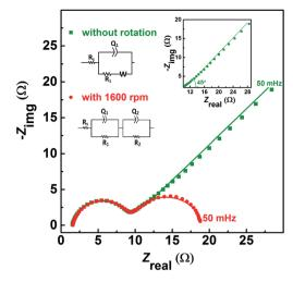
Fig. 2 EIS patterns recorded at EP on carbon-modified GCE without rotation and with 1600 rpm in equimolar (0.2 M) concentration of V $^{4+}$  and V $^{5+}$  in 3 M H $_2$ SO $_4$  electrolyte. The symbols and solid lines show the experimental and the fitted data, respectively. The corresponding ECs are shown in the insets. The expanded view of the  $45^\circ$  line is shown in the inset.
