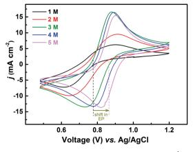
Fig. 8 CVs recorded on carbon-modified GCE at 20 mV s $^{-1}$  scan rate in equimolar (0.2 M) solution of V $^{4+}$  and V $^{5+}$  in H<sub>2</sub>SO<sub>4</sub> electrolyte of different concentrations. The dotted lines show the shift in EP with supporting electrolyte (H<sub>2</sub>SO<sub>4</sub>) concentration.
