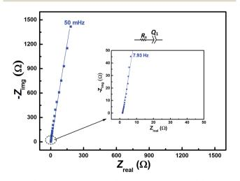
Fig. 3  $\,$  EIS patterns recorded at OCP on carbon-modified GCE without rotation in 0.2 M V<sup>5+</sup> in 3 M H<sub>2</sub>SO<sub>4</sub> electrolyte.
