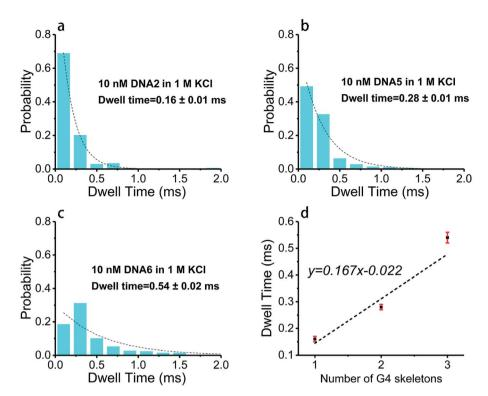
Fig. 5 Nanopore translocation duration of G4 recorded with 100 nM DNA2, DNA5 and DNA6, performed in 1 M KCl, 10 mM Tris, 1 mM EDTA at pH 7.4 under 200 mV bias voltage in an  $\sim$ 4.2 nm nanopore. (a–c) Histograms of dwell time with exponential decay fitting curves; all the data were treated with the same bin size of 0.2 ms. (d) Line fitting graph of dwell time as a function of the number of G4 skeletons.
