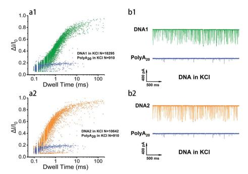
Fig. 2 Discriminative analysis of G4 translocation properties. (a1 and a2) Scatter plots showing event distribution of G4 folded with 100 nM of telomeric DNA1, DNA2 and polyA $_{20}$  in 1 M KCl, 10 mM Tris, 1 mM EDTA at pH 7.4 with  $\sim$ 3.2 nm nanopores under 200 mV external voltage. (b1 and b2) Representative translocation current traces of indicated DNA during 2 s.
