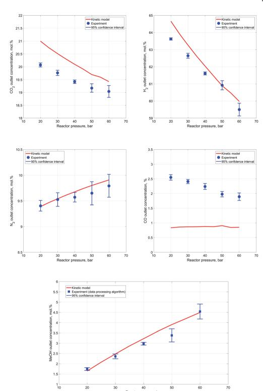
Fig. 7 (a). Dependence of the outlet  $CO_2$  concentration from the reactor pressure. (b) Dependence of the outlet  $H_2$  concentration from the reactor pressure. (c) Dependence of the outlet  $N_2$  concentration from the reactor pressure. (d) Dependence of the outlet CO concentration from the reactor pressure. (e) Dependence of the outlet MeOH concentration from the reactor pressure.
