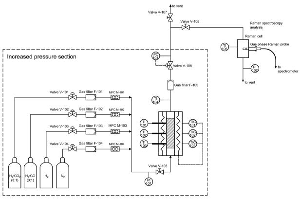
Fig. 1 Flowchart of the reactor system.
