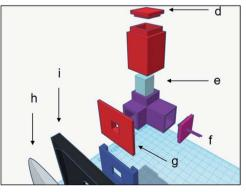
Fig. 3 Details of each part of the proposed 3D printable device. Dark cover (a), cuvette holder (b), sliding support (c), top of dark cover (d), cuvette (e), LED light and press-in cover (f), movable slide (g), smartphone (h), plastic phone case (i). The color of the images is illustrative.
