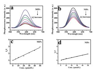
Fig. 10 (a) The RTP emission spectra of Mn-doped ZnS QD@ms-MIPs (30 mg  $L^{-1}$ ) and (b) Mn-doped ZnS QD@ms-NIPs (30 mg  $L^{-1}$ ) with the addition of different concentrations of phenol in DDW. The Stern–Volmer values for (c) Mn-doped ZnS QDs@ms-MIPs and (d) Mn-doped ZnS QDs@ms-NIPs.
