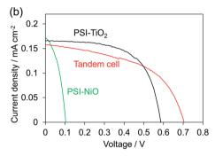
Fig. 4 (a) Schematic representation of the tandem cell power generation mechanism. (b) J-V curves under AM 1.5G (100 mW cm<sup>-1</sup> of the tandem cell and individual n- and p-biophotovoltaic cells
