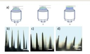
Fig. 2 (a) Length adjustment scheme. (b-d) Microneedle (MN) micrographs when using 50, 100, and 150 µL of spacer.
