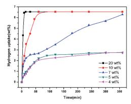
Fig. 4 Influence of catalyst dosage proportions on the hydrogenation of 8-MQL. General reaction conditions: 4 g 8-MQL, 40 ml dioxane as solvents, 160 °C, 7 MPa H<sub>2</sub>.
