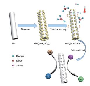
Fig. 1 Schematic of the preparation process of GF@P electrode.
