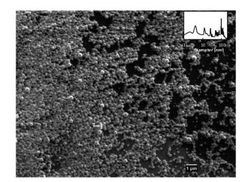
Fig. 7 Scanning electron micrograph of PLGA nanoparticles.
