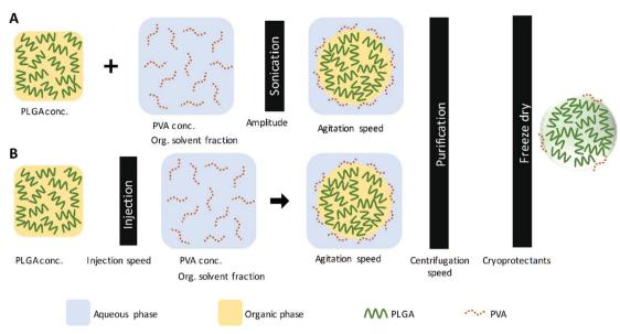
Fig. 1 Nanoparticle preparation scheme by (A) the single emulsification and (B) the nanoprecipitation techniques.
