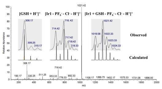
Fig. 1 ESI-MS spectrum with the isotopic distribution of the solution sample from the reaction of Ir1 (1 mM) and GSH (10 mM) in CH<sub>3</sub>OH/H<sub>2</sub>O (v/v, 1:1) after incubation for 6 h at 310 K. The assignments for the peaks are listed in the inset.
