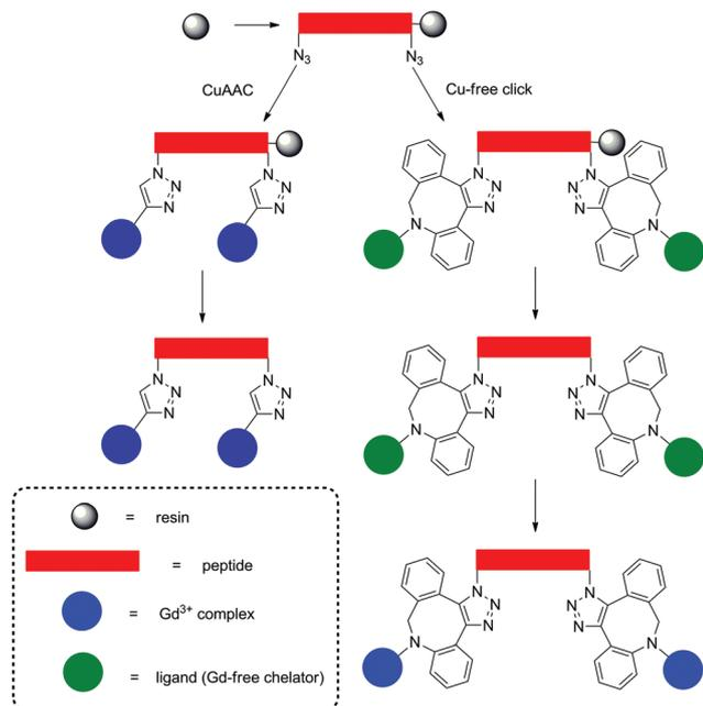
**Fig. 6** Illustration of SPS click chemistry approaches employed in CA development. The approaches include attaching  $\text{Gd}^{3+}$  complexes directly to the resin using CuAAC (left) or attaching Gd-free chelators using Cu-free click chemistry before complexing post cleavage.
