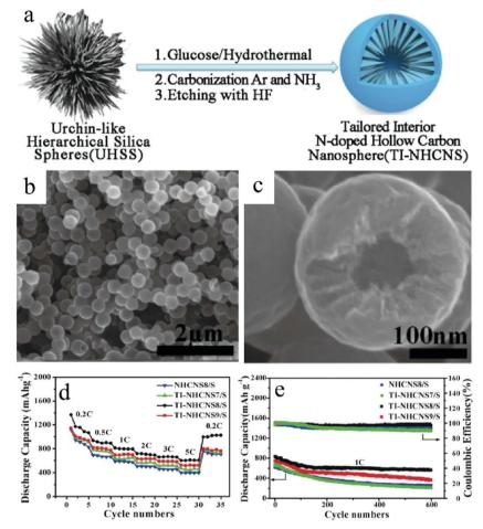
**Fig. 15** (a) Fabrication processes of N-doped hollow carbon nanospheres with a tailored internal structure (TI-NHCNS). (b and c) SEM images of TI-NHCNS8 at different magnifications. (d) Rate and (e) cycling performance of the as-prepared TI-NHCNS/S cathodes. Reproduced with permission.<sup>48</sup> Copyright 2020, Wiley-VCH.
