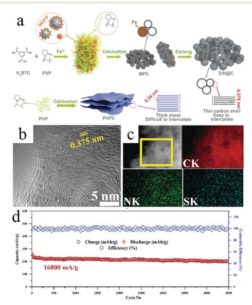
Fig. 18 (a) Schematic representation of S/N@C synthesis. (b) HRTEM and (c) HAADF analysis of S/N@C. (d) Cycling performance at a current density of 16 000 mA  $g^{-1}$ . Reproduced with permission.<sup>57</sup> Copyright 2019, Wiley-VCH.
