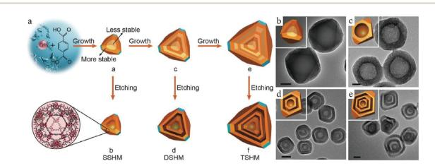
Fig. 11 (a) Fabrication of single-, double-, and triple-shelled hollow MIL-101, which are denoted as SSHM, DSHM, and TSHM, respectively. TEM images of (b) solid MIL-101, (c) SSHM, (d) DSHM, and (e) TSHM. Reproduced with permission.<sup>38</sup> Copyright 2017, Wiley-VCH.
