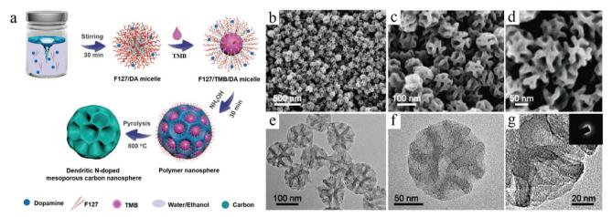
**Fig. 6** (a) Synthesis procedure for the dendritic N-doped mesoporous carbon nanospheres prepared by the versatile nanoemulsion assembly approach. (b–d) SEM and (e and f) TEM images of the dendritic N-doped mesoporous carbon nanospheres with ultralarge pore size prepared by the versatile nanoemulsion assembly approach. Reproduced with permission.<sup>17b</sup> Copyright 2019, American Chemical Society.
