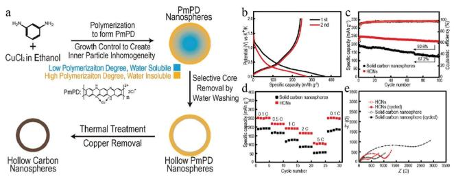
**Fig. 20** (a) Synthesis protocol for HCNs. (b) First two charge/discharge curves for HCNs at 0.1C. (c) Cycling performance and (d) rate capability of two samples, namely, HCNs and solid carbon nanospheres. (e) Electrochemical impedance of the two samples before cycling and after 100 cycles. Reproduced with permission.<sup>36</sup> Copyright 2020, American Chemical Society.
