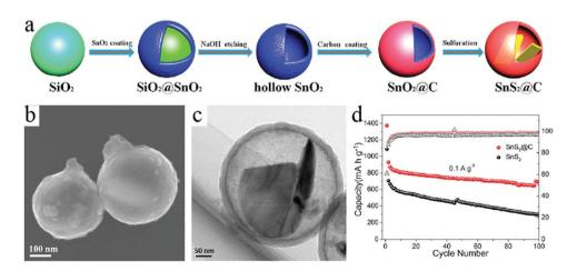
Fig. 19 (a) Schematic of the formation process of  $SnS_2@C$ . (b) SEM and (c) TEM images of the as-prepared  $SnS_2@C$ . (d) Cycling performance of  $SnS_2@C$  electrode at current densities of 0.1 A g<sup>-1</sup>. Reproduced with permission.<sup>61</sup> Copyright 2018, Elsevier.
