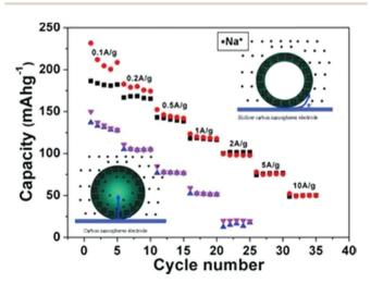
**Fig. 17** Schemes of the electrochemical reaction process and realistic rate performance of HCNs and solid carbon spheres. Reproduced with permission.<sup>55</sup> Copyright 2012, Wiley-VCH.
