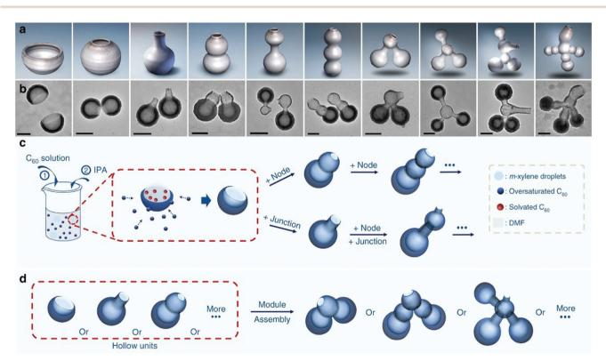
**Fig. 7** Schematic illustrating the concept and design. (a) Models of pottery and (b) TEM images of their corresponding nanostructures created with nanopottery. (c) Schematics illustrating the synthesis of different hollow units and (d) connections between the hollow units. Reproduced with permission.<sup>32</sup> Copyright 2019, Nature.
