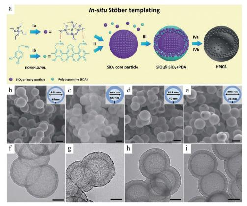
**Fig. 2** (a) Schematic illustration of the *in situ* Stöber templating of HMCS. (b–e) SEM and (f–i) TEM images of HMCSs with different core–shell sizes for different concentrations and addition times of dopamine. Reproduced with permission.<sup>24a</sup> Copyright 2016, Royal Society of Chemistry.
