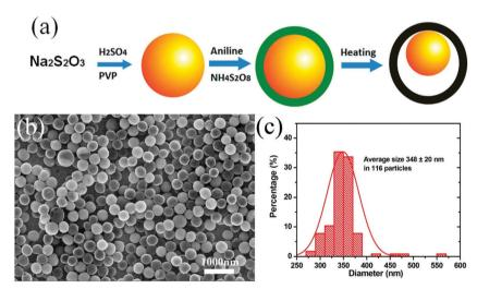
**Fig. 3** (a) Two-step synthesis route for the S–PANI composite; the yellow sphere represents sulfur; dark green shell, PANI; and black shell, vulcanized PANI. (b) SEM images of the S–PANI core–shell composite using  $H_2SO_4$  as the acid source and (c) the particle size distribution. Reproduced with permission.<sup>25</sup> Copyright 2013, American Chemical Society.
