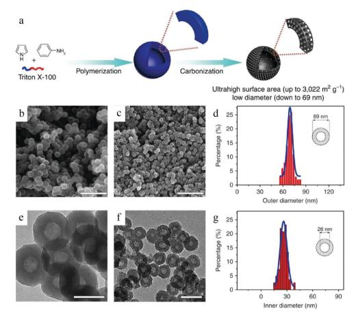
**Fig. 5** (a) Schematic illustration of the preparation of HCNs. SEM images of (b) polyaniline-*co*-polypyrrole (PACP) and (c) HCN-900-20H2R. TEM images of (e) PACP and (f) HCN-900-20H2R. Histograms of the (d) outer and (g) inner diameters of HCN-900-20H2R as per the analyses of the SEM and TEM images, respectively. Reproduced with permission.<sup>36</sup> Copyright 2015, Nature.
