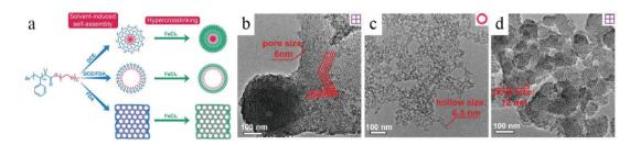
**Fig. 9** (a) Synthesis route of hypercrosslinked polymers (HCPs) with different morphologies. TEM images of mesoporous bulk HCPs synthesized with (b) PEO45-*b*-PS190, (c) HCPs synthesized with PEO45-*b*-PS190, and (d) mesoporous bulk HCPs synthesized with PEO117-*b*-PS307. Reproduced with permission.<sup>34</sup> Copyright 2019, Wiley-VCH.
