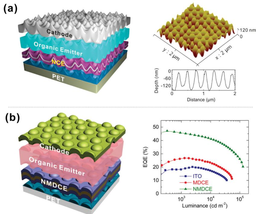
**Fig. 17** (a) Schematic illustration of flexible OLEDs using a nanostructured composite electrode and the AFM profile of imprinted UV-resin layer with quasi-random nanostructures. Reproduced with permission from ref. 205. Copyright 2016 Optical Society of America. (b) Flexible OLED structure with a nanopatterned metal-dielectric electrode on a plastic substrate and EQE values as a function of luminance. Reproduced with permission from ref. 206. Copyright 2015 American Chemical Society.
