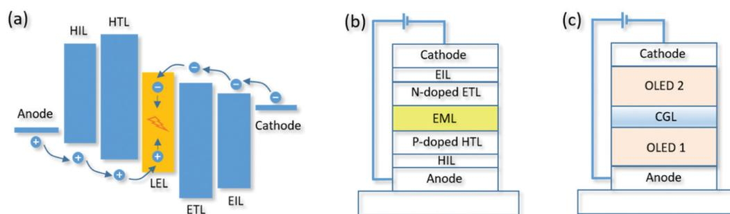
Fig. 4 Representative device architectures of OLEDs. (a) The working mechanism of OLEDs, (b) charge injection and transport in OLEDs enhanced by p- and n-type electrical doping, and (c) tandem OLED structures with stacked emission units connected by a charge generation layer (CGL).
