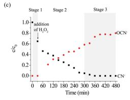
Fig. 9 Reversible detection of cyanide by **15** via the degradation of newly formed "receptor–cyanide ensemble", i.e.  $[Cu^{II}(CN)_4]^{2-}$ , under the ICDA.
