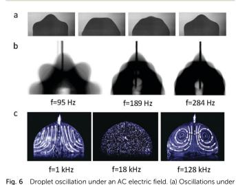
60 V and 180 Hz. Snapshots are 1 ms apart. (b) Various modes of oscillation under different resonance frequencies. (c) Rapid hydrodynamic flow was observed with f = 1 kHz. No hydrodynamic flow occurred with f = 18 kHz, and a distinct type of flow was observed when f = 128 kHz.
