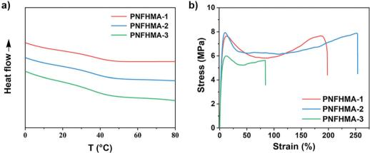
Fig. 5 (a) DSC and (b) stress-strain curves of UHMW fluoropolymers with different  $M_{\rm n}$ . Red line, PNFHMA-1,  $M_{\rm n}=6.72\times10^5$  Da, D=1.18; blue line, PNFHMA-2,  $M_{\rm n}=1.88\times10^6$  Da, D=1.12; green line, PNFHMA-3,  $M_{\rm n}=3.20\times10^6$  Da, D=1.09.
