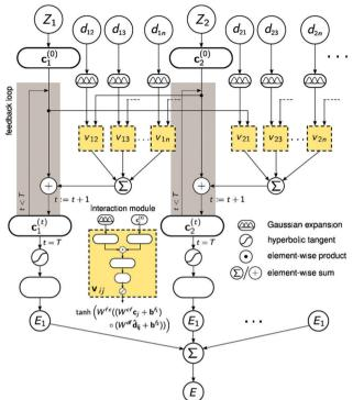
Fig. 7 The architecture of SchNet.<sup>39</sup> The iteration loop implements eqn (1), and the interaction module (a neural network) implements eqn (2).
