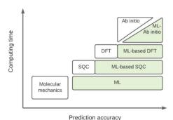
Fig. 3 Schematic representation of quantum chemical and ML approximations with respect to computational cost and accuracy, which generalises the literature.<sup>24</sup> DFT = density functional theory; SQC = semi-quantitative quantum chemistry.
