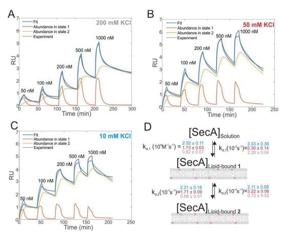
Fig. 1 Interaction of SecA with acidic phospholipids containing membranes. (A) Surface plasmon resonance experiments of SecA binding to a supported lipid bilayer made of *E. coli* lipids examined at a KCl concentration of 200 mM. Fit (blue line) represents the sum of abundances in state 1 and 2. (B) As in (A) but at 50 mM KCl. (C) As in (A) but at 10 mM KCl. (D) Sketch of the two state model that best fit the SPR sensorgrams.
