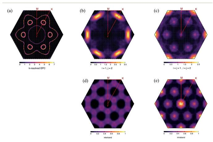
Fig. 6 k-Resolved EPC constant ( $\lambda_k$ ) on the Fermi surface at -5.5% strain (a),  $\lambda_{a\nu}$  from interband scattering (b),  $\lambda_{a\nu}$  from intraband scattering (c), nesting function constructed from  $d_{xy}$ ,  $d_{x_2-y_2}$  and  $d_{z_2}$  orbital of Mo atoms extracting the contribution from different band indexes (interband) (d), and the same band index (intraband) (e). The nesting functions were normalized to the same scale with 1.0 as the maximum of comparison.
