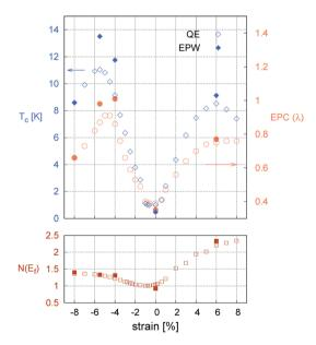
Fig. 3 Change in transition temperature  $T_c$  [K], EPC constant ( $\lambda$ ), and DOS at the Fermi level ( $N(\varepsilon_{\rm F})$ ) [states/spin/eV/unit cell] as a function of strain. Opened and closed dots refer to converged values in coarse kand q-meshes from Quantum Espresso and in dense k- and q-meshes from EPW, respectively. Both results indicated well-converged conditions.
