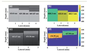
Fig. 1 Simulated (a) OCT (present submicron scale structure mentioned) (b) nsOCT (detected submicron scale structure with colour bar), experimental (c) OCT (present submicron scale structure mentioned), (d) nsOCT (colour bar represents detected submicron scale structure).
