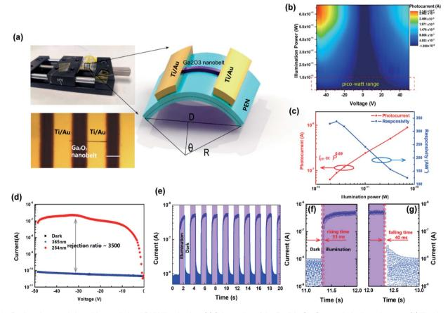
Fig. 2 Device characteristics with unpolarized DUV illumination. (a) Schematics of the flexible  $Ga_2O_3$  nanobelt photodetector. (b) Illumination—power-dependent I-V characteristics. (c) Diagram of photocurrent and responsivity *versus* illumination power. (d) Photocurrent under UV254 nm irradiation compared with that under UV365 nm irradiation. (e) Time-resolved photoresponse characteristics with V=50 V. (f) Rising and (g) falling edge of one photoresponse cycle.
