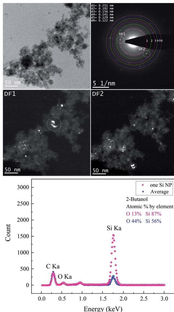
Fig. 6 The femtosecond laser-synthesized Si nanoparticles in 2-butanol. ( $N = 1000$ ,  $F = 4.42 \text{ J cm}^{-2}$ ). The BF-TEM image (upper left), SAED pattern (upper right) and the DF-TEM images related to different diffracted electron beams along the 1<sup>st</sup> and 2<sup>nd</sup> ring. The EDX spectrum of several Si NPs shown in the BF-TEM and that of one single Si NP.
