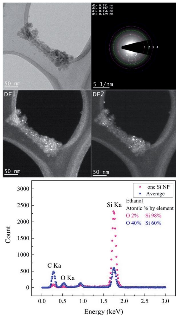
Fig. 4 The femtosecond laser-synthesized Si nanoparticles in ethanol. ( $N = 1000$ ,  $F = 4.90 \text{ J cm}^{-2}$ ): BF-TEM image (upper left), SAED pattern (upper right) and DF-TEM images related to different diffracted electron beams along the 1<sup>st</sup> ring. The EDX spectrum contains an average of several Si NPs and one of a single Si NP.
