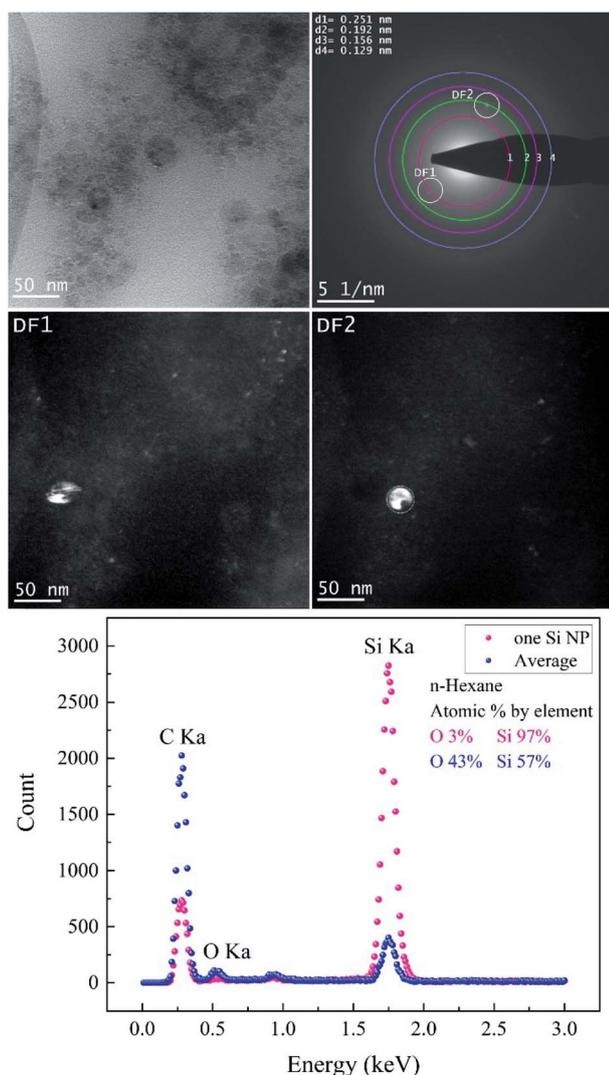
Fig. 7 The femtosecond laser-synthesized Si nanoparticles in *n*-hexane. ( $N = 1000$ ,  $F = 10.46 \text{ J cm}^{-2}$ ). The TEM bright-field image, SAED pattern (upper right) and dark-field images related to different diffracted electron beams along the 1<sup>st</sup> and 2<sup>nd</sup> ring. The EDX spectrum from several small Si NPs and one Si NP.
