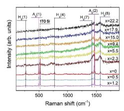
Fig. 9 Raman spectra of the Au<sub>x</sub>C<sub>60</sub> films with different Au concentrations (x). The x values are shown for the respective spectra. Some of the  $C_{60}$  vibration modes with  $A_a$  and  $H_a$  symmetry are indicated by vertical lines. The position of the intense 1TO Si(100) mode is indicated by the dashed vertical line (see text).
