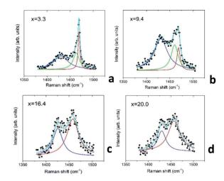
Fig. 10 Raman spectra of the  $Au_xC_{60}$  mixture films near the positions of the  $H_g(7)$  and  $A_g(2)$  modes of  $C_{60}\!\colon$  (a and b) the mixture films from the interval R2; (c and d) the mixture films from the interval R3. The experimental spectra (black dots) fitted by a superposition of Lorentzians (light-blue line). See description in the text.
