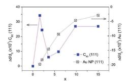
Fig. 8 The relative change of lattice parameter in fcc- $C_{60}$  (blue boxes) and in fcc-Au NPs (crossed circles) upon increase of Au concentration x in the  $Au_xC_{60}$  mixture films.
