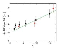
Fig. 7 Dependence of the Au NP size (2R, here R is the spherical NP radius) on the Au concentration (x) in the Au $_x$ C $_{60}$  mixture films as obtained from the TEM analysis (red stars) and from the Scherrer analysis of the XRD line-broadening (black circles).
