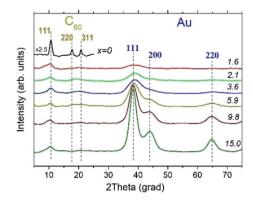
Fig. 6 XRD patterns of pure  $C_{60}$  film (x=0) and of  $Au_xC_{60}$  mixture films with different Au contents (x). The x values are shown in the plots. Experimental XRD patterns were smoothed prior to plotting, and the rapidly increasing background at smaller angles was subtracted.
