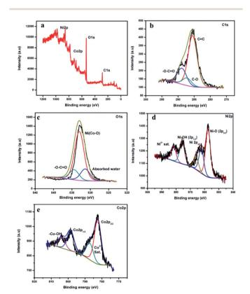
Fig. 4 (a) XPS survey spectra of NiCo-MOF/NF, and (b-e) C 1s, O 1s, Ni 2p and Co 2p high resolution spectra, respectively.
