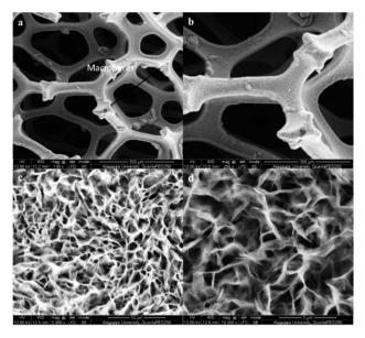
Fig. 2 FE-SEM images of NiCo-MOF/NF at various scales: (a) 500 μm, (b) 300  $\mu$ m, (c) 10  $\mu$ m, and (d) 5  $\mu$ m.
