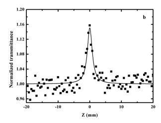
Fig. 2 Representative "open-aperture" Z-scan curves obtained for the oven annealed samples using 600 fs laser pulses at (a) 1030 nm, I = 2 GW cm<sup>-2</sup> and (b) 515 nm, I = 2 GW cm<sup>-2</sup>.
