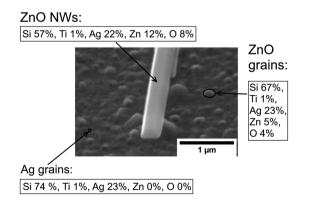
Fig. 8 SEM image of ZnO NWs grown on Ag (45  $^{\circ}$ C tilted) at a precursor concentration of 5 mM and growth time of 18 hours. EDX data (elemental percentage) have been shown at the points of ZnO NWs, ZnO grains, and Ag grains. The electron beam penetration depth is  $\sim$ 1  $\mu$ m; carbon and other contaminants have been ignored.
