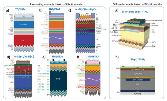
Fig. 4 Representative examples of the successful RJs used in literature for passivating contacts and diffused-junction contacts based c-Si bottom cells (References:  $a_s^{55}$   $b_s^{56}$   $c_s^{49}$   $d_s^{33}$   $e_s^{57}$   $f_s^{58}$   $g_s^{59}$   $h^{60}$  reprint with permissions).
