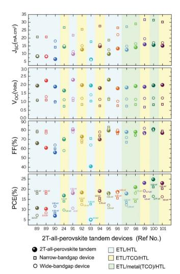
Fig. 7 Photovoltaic device characteristics of tandem devices and individual subcells in literature for 2-terminal all-perovskite tandems, as summarized in Table 3 and are classified according to the structure of the RJ layer. (Spheres, squares, and hollow circles correspond to the champion parameters of the tandem device, the narrow-bandgap topcell and the wide-bandgap bottom-cell employed in the reports, respectively.)
