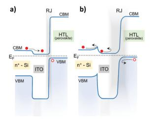
Fig. 3 Band diagram of the RJs of the silicon/perovskite tandems with (a) ideal and (b) with Fermi level pinned contacts.
