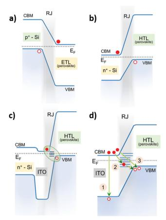
Fig. 2 Band diagrams of the RJ in silicon/perovskite tandems. (a) and (b) General cases of p-i-n and n-i-p tandems based on the perovskite top cell configuration. (c) Band diagram of the ITO-assisted RJ. (d) Zoom-in of panel c that represents the recombination mechanisms at the ITO/perovskite HTL interface for a p-i-n tandem
