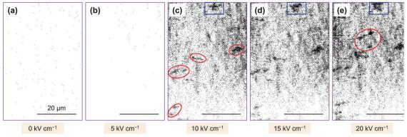
Fig. 3 A dramatic change of the Kerr image was observed between 5 kV cm<sup>-1</sup> and 10 kV cm<sup>-1</sup>. The red circles in (c) and (e) highlight newly reversed domains generated by the applied electric field, and the blue square highlights the electric-field-driven domain expansion. Note that the tiny dark spots are caused by noise.
