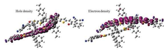
Hole and electron density distribution relative to the triplet  $T_5$  excited state in an ITIC dimer which shows a strong CT character.
