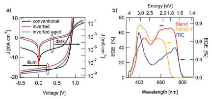
Fig. 2 Solar cell characteristics. (a) J-V-curves of PBDB-T:ITIC solar cells in dark and under illumination: conventional (black traces), inverted (red) and aged inverted (blue). (b) EQE spectra for inverted solar cells (red trace) together with diodes from pure PBDB-T (yellow) and pure ITIC (blue).
