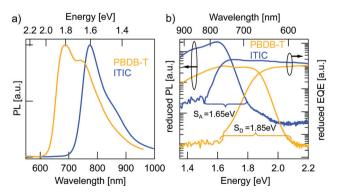
**Fig. 3** Determination of the singlet excited state energies of pure materials. (a) PL spectra of pure material films: PBDB-T (yellow) and pure ITIC (blue). (b) The same PL data represented as reduced PL/E together with reduced EQE  $\times$  E of diodes of the pure materials in logarithmic representation. The onsets of PL and EQE are marked, as well as their midpoint as an estimate for the singlet energy.
