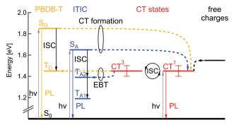
Fig. 5 Jablonski diagram of the PBDB-T:ITIC blend.  $S_D$ ,  $T_D$  – singlet and triplet excited states of the donor PBDB-T (yellow).  $S_{Ar}$   $T_{A\underline{1}}$ ,  $T_{A2}$  – singlet and two triplet states of the acceptor ITIC (blue). CT<sup>1</sup>, CT<sup>3</sup> - singlet and triplet charge transfer states (red), ISC - intersystem crossing, EBT electron back transfer.
