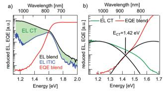
Fig. 4 Determination of CT state energy. (a) Reduced EQE  $\times$  E spectrum for an inverted BHJ solar cell (red) together with EL/E spectra for the same solar cell (black trace) and an ITIC diode (blue). The green shaded area represents the CT EL emission. (b) Subtracted solar cell EL/E spectrum (green) and reduced EQE  $\times$  E spectrum (red) together with Gaussian fitting curves (black) to determine  $E_{CT}$ .
