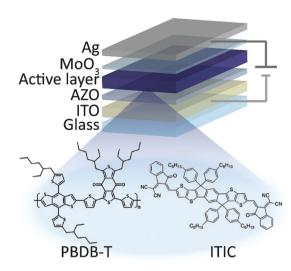
Fig. 1 Structure of inverted solar cells.
