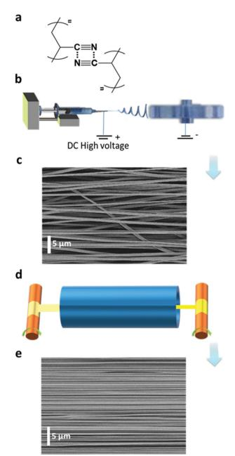
Fig. 1 Fabrication process and microstructure of ENRs. (a) Chemical structure of PAN with dipole-dipole attraction interactions. (b) Electrospinning setup. (c) A SEM image of the PAN as-spun ENRs. (d) Roll-to-roll heat-stretching setup. (e) A SEM image of the PAN ENRs after the heatstretching process with a stretch ratio of six.
