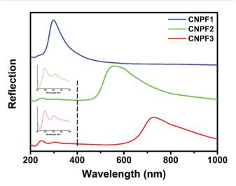
Fig. 3 UV-Vis spectra of CNPF1-3 at normal incidence with varying photonic-photonic coupling. The inset shows the magnified UV spectra of CWF2 and 3 at a short wavelength (200-400 nm) which highlights the surface grating induced double-peak spectra.
