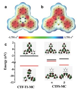
Fig. 13 Elemental doping on CPPs for controlling the energy band structure. Charge distributions of cluster models from structures of (a) covalent triazine framework (CTF-T1-MC) and (b) sulfur-doped CTF (CTFS-MC), (c) The calculated HOMO/LUMO orbitals of the cluster models. Adapted with permission. 106 Copyright 2016 The Royal Society of Chemistry.
