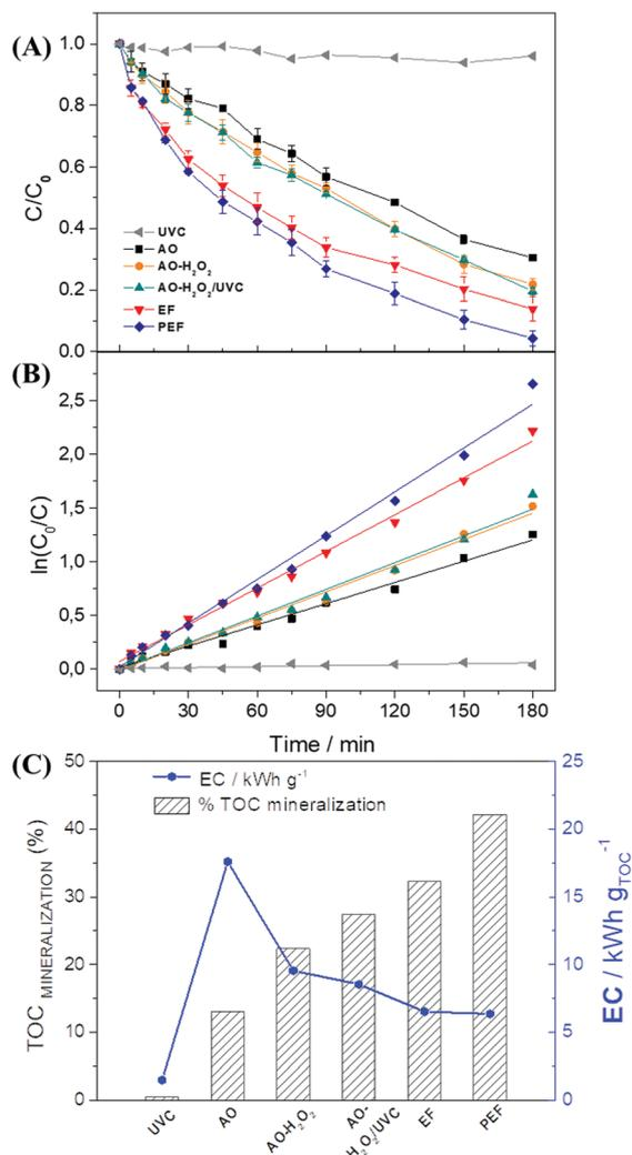
Fig. 5 (A) Effect of different AEOPs on PRM degradation in 180 min of experiment at  $j = 75 \text{ mA cm}^{-2}$  using the 1.0% NQE modified GDE with  $0.1 \text{ mol L}^{-1} \text{ K}_2\text{SO}_4$  under pH 2 and 0.2 bar of  $O_2$  flow; (B) analysis of the pseudo-first order kinetics; and (C) comparison between the TOC mineralization and energy consumption in each system.
