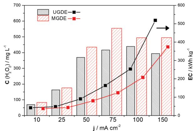
Fig. 4 Comparison of the maximum concentration of  $\text{H}_2\text{O}_2$  electrogenerated in 120 min on the unmodified GDE (UGDE) and modified GDE (MGDE) with the respective energy consumption for the UGDE and MGDE, calculated based on eqn (10).
