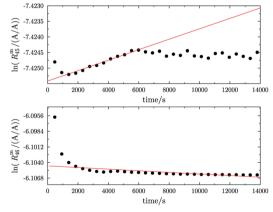
(c) Logarithms of  $R_{45}^{\rm m}$  and  $R_{46}^{\rm m}$  against time during the measurement of parent material A. Prior to the measurement, an aliquot of the gas was filled in one of the gas spheres. Previous to the filling with gas A, a platinum band was placed into the sphere. Subsequently, the sphere was heated for 39.5 h with a
