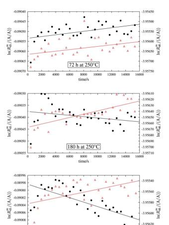
Fig. 2 Heating history of blend b1. Top:  $\ln(R_{45}^m)$  (black dots) and  $\ln(R_{46}^m)$  (red triangles) against time after heating at 250 °C for 72 h. Centre:  $\ln(R_{45}^m)$  and  $\ln(R_{46}^m)$  against time after heating at 250 °C for 180 h. Bottom:  $\ln(R_{45}^m)$  and  $\ln(R_{46}^m)$  against time after heating at 250 °C for 600 h. Mind the different scales.
