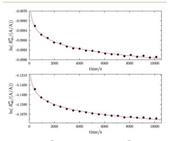
Fig. 1 Plot of  $\ln(R_{45}^{\rm m})$  against time (top) and  $\ln(R_{46}^{\rm m})$  against time (bottom) in case of blend b1. The black dots are the measured ratios, the red lines are fits using the generic equation  $\ln(R_x^{\rm m}) = a_1 \times \ln(t) + a_0$ . Both graphs show that the ln of both ratios does not linearly increase over time.
