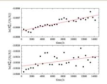
(a)  $\ln(R_{45}^m)$  against time (top) and  $\ln(R_{46}^m)$  against time of blend b1 (bottom). The blend was heated with a Bunsen burner for 20 min before the measurement. The red line in both graphs indicates a linear fit.
