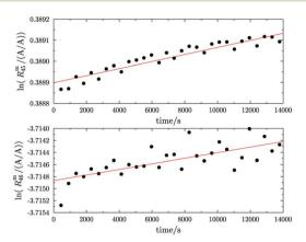
(a)  $\ln(R_{45}^{\rm m})$  against time (top) and  $\ln(R_{46}^{\rm m})$  against time of blend b2 (bottom). The blend was heated with a Bunsen burner for 5 h before the measurement. The red line in both graphs indicates a linear fit.
