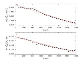
(a) Logarithms of  $R_{45}^{\rm m}$  (top) and  $R_{46}^{\rm m}$  (bottom) against time during the measurement of parent material A (12C enriched material). The gas was heated prior to the measurement for 25 h with a Bunsen burner ( $\vartheta \approx 1800$  °C).
