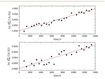
Fig. 8 Logarithms of  $R_{45}^{m}$  (top) and  $R_{46}^{m}$  (bottom) against time during the measurement of parent material B (13C enriched material). The gas was heated prior to the measurement for 13 h using a Bunsen burner ( $\vartheta$ ≈ 1800 °C).
