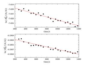
(b) Logarithms of  $R_{45}^{\rm m}$  and  $R_{46}^{\rm m}$  against time during the measurement of parent material A. Prior to the measurement, an aliquot of the gas was filled in one of the gas spheres and heated for 48 h with a Bunsen burner ( $\vartheta \approx 1800 \,^{\circ}\text{C}$ ). (Six outliers were removed.)
