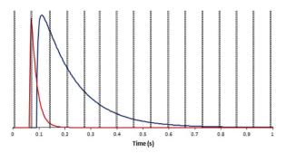
Fig. 4 Model  $^{235}$ U IC signal response (red) and  $^{238}$ U Faraday detector signal response (blue) for the DCI: created with the determined exponential Gaussian hybrid functions, values every 3 ms. Blind time events (black dotted box) denote an example 66 ms integration time. The proportion of total counts lost to blind time differs between the IC and Faraday signal responses.
