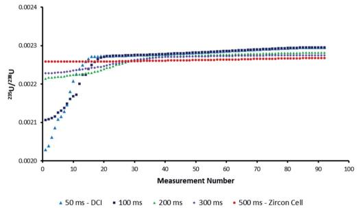
Fig. 6 Plot of possible uncorrected  $^{235}$ U/ $^{238}$ U isotope ratios for the average model pulse due to the influence of blind time. The 100–300 ms datasets were created by widening the model IC pulse *via* changes to the parameters in the exponential-Gaussian hybrid function. As the pulse duration increased, the impact of blind time on isotope ratio accuracy was reduced.
