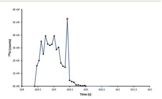
Fig. 7 235U pulse profile of the ablation of a NUSIMEP-6 particle, Zircon Cell. The standard profile is interrupted by a large single integration spike in the signal.
