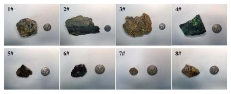
Fig. 1 Photos of eight uranium ore samples of different origins. The coin for comparison is 25 mm in diameter.
