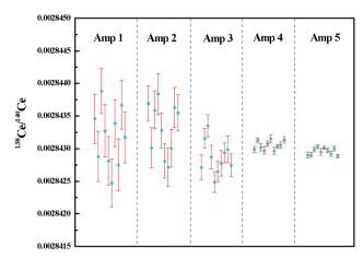
Fig. 5  $^{138}$ Ce/ $^{140}$ Ce ratios measured for 2  $\mu$ g JMC-304 using different combinations of amplifiers with the FPIE method as Ce $^+$ . The error bars in each measurement are given in 2SE. Amp 1–5 refer to different combinations of amplifiers in the Faraday cup configuration listed in Table 5.
